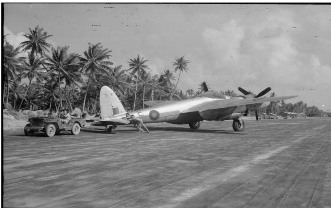
*De Havilland Mosquito PR Mark XXXIV, RG203 'E', of No. 684 Squadron RAF Detachment is towed into position for takeoff at Brown's West Island, Cocos Islands in June 1945. Note the unusual camouflage with azure blue lower surfaces, and silver upper surfaces. Thirty eight sorties were flown by 684 SQN from the Cocos Islands. The PR.XXXIV variant carried additional fuel in a bulged bomb bay tank, yielding a Combat radius of ~1500 NMI. (IWM Photograph)*
